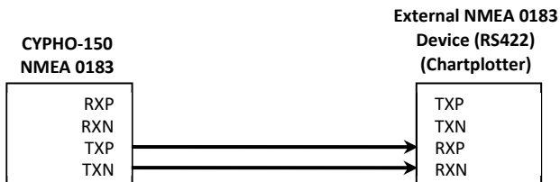
Figure 8 NMEA 0183 Connection illustration
