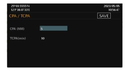
To save the setting, select the SAVE button in the view and press —. The system will ask whether the changes should be saved. Select YES to save or NO to discard and return to AIS settings submenu.
