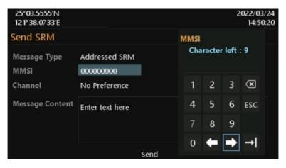
After entering the MMSI number, choose the **Channel**. It gives you the option to send message through channel A, B or Both A & B. By No Preference, which is the default option, the system will select the channel automatically. Then, compose the message.
