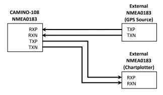
Figure 6 NMEA 0183 Multiplexing Connection
