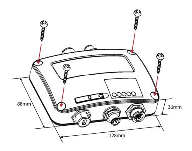
Figure 1 Mounting the transponder
