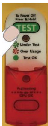
Figure 12 Testing of AIS SART
