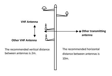
Figure 5 VHF Antenna Installation
