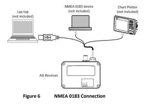
The figure below describes how to wire your AIS receiver with NMEA 0183 devices and power source.
